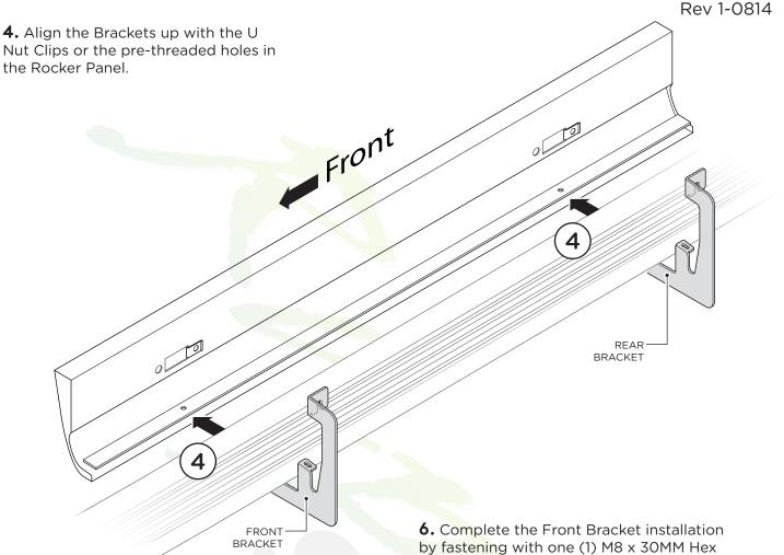
**5.** Fasten the lower portion of the Front Bracket using one (1) M8 Flange Lock Nut, one (1) Weld Support, one (1) Nylon Washer and one (1) M8 X 30MM Hex Head Bolt. Repeat for Rear Bracket.
