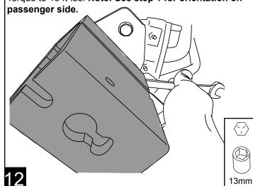
Set step pad into center position and tighten screws. Tighten to 5 ft-lbs.
