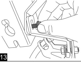
Set frame mount into position and tighten two bolts. Torque to 16 ft-lbs. Note: See step 1 for orientation on
