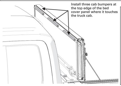
Clean the surface where the bumpers will go with soap and water to remove dirt and debris. Then clean the same surface with isopropyl alcohol to remove wax or grease and to evaporate any remaining water. Allow the surface to dry.
