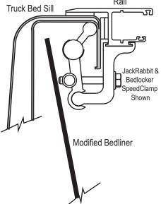
The Pace Edwards Rails lay flat on the bed sill and the clamps clamp to the bed sill, this makes it necessary for the bedliner to be pushed to the backside of the sill.
