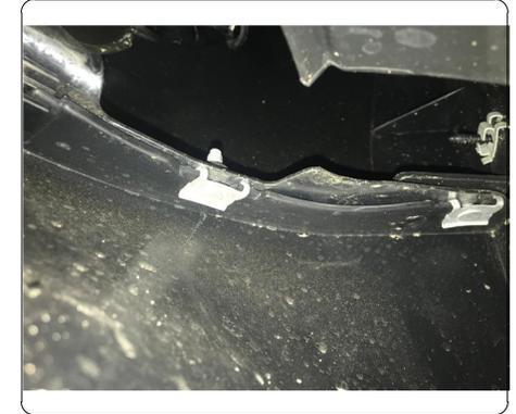
2. If present, remove tow hooks and return to owner. Insert (1) 1/2" carriage bolt and (1) CM-SP10 through front of vehicle cabin, on both sides, using provided through holes.
