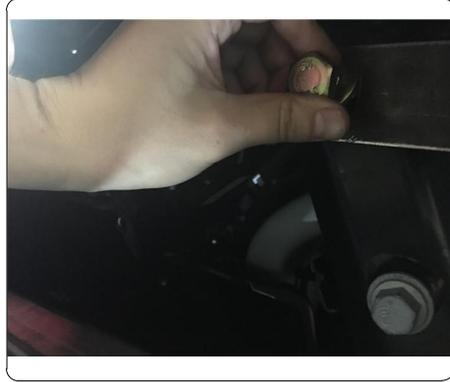
5. Trim lower fascia using trim diagram as a reference. Reinstall trimmed fascia.
