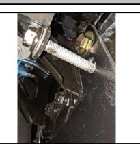
4. Align the lower mounting holes on sideplates with the vehicle mounting holes and insert a 7/16" carriage bolt and spacer into the mounting holes. Finish securing the hitch to the vehicle using the 7/16" serrated flange nuts.
