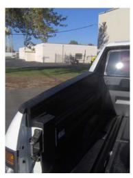
**Step 3:** Insert Advantage Bolts into proper Holes. Tighten with keys provided.
