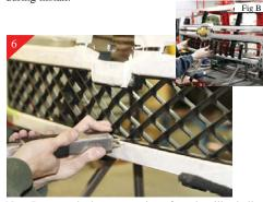
Next Remove the bottom section of stock grille shell following the same procedure as the upper. Again using an air saw or other cutting devise cut all vertical and horizontal attachment points of top section where it meets the outer shell.
