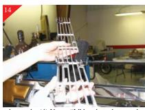
Next locate the (4) Upper "L" brackets that attached to top portion of the billet grille. Place supplied u-clips on long end of the brackets and attach long end to the billet grille. Now locate the (2) small "L" brackets and place u-clip on the long end and attach to billet grille using 10-24 x 1" bolts.
