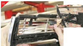
Using a scribe mark the hole locations to be drilled.
