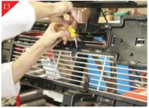
Attach steel bracket using the supplied sheet metal screws.
