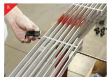
Place the bottom billet grille on a protective work surface. Next locate (4) brackets that attach to bottom portion of the billet grille. Place supplied u-clips on the long end of the brackets as shown. Now using the 10-24 x 1" bolts attach brackets to billet grille.
