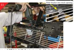
Using a 1/8" bit drill the just marked hole locations. Place billet grille back into opening. Next locate the (2) small steel brackets and place supplied u-clips on the hole end of the brackets and attach to billet grille. Note that the bracket slides into a stock opening. Still using the 1/8" bit drill just through steel bracket as shown above.
