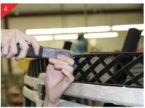
Using an air saw or other cutting devise cut all vertical and horizontal attachment points of top section where it meets the outer shell.
