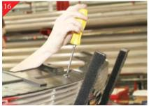
Attach top (4) bracket using the supplied 10-24 x 1" bolts, fender washers and u-clips. Double check all fasteners. Reattach stock grille shell on vehicle.
