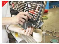
Attach bottom brackets using the supplied 10-24  $\rm x$  1" and u-clips. Place the u-clip on the under side of grille shell and attach.
