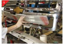
Now place bottom billet grille into opening and center. Be sure to align billet grille into opening and make sure grille is flush with opening.
