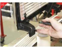
Again making sure the billet grille in flush with the opening. Use a scribe and mark the hole locations for drilling. After marking remove billet grille.
