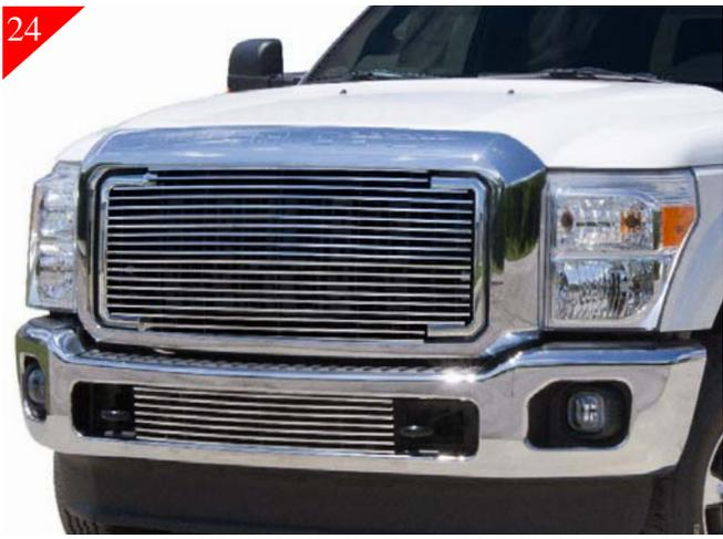
After billet grille is attached check alignment make any necessary adjustments by loosening the bolts slightly make adjustment and tighten in place. Tighten all hardware. Reattach shell back on vehicle.
