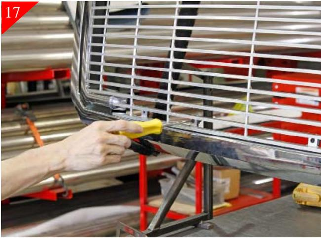
After attaching all bottom brackets to the grille shell, place billet grille back into opening center and attach billet grille to the 2 center bottom brackets. This will hold the billet grille in place while marking hole locations for the upper brackets.
