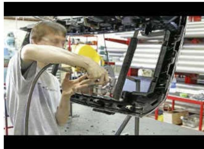
10 After removing center sand all cut areas using a sanding block or power sander. Double click for playback.
