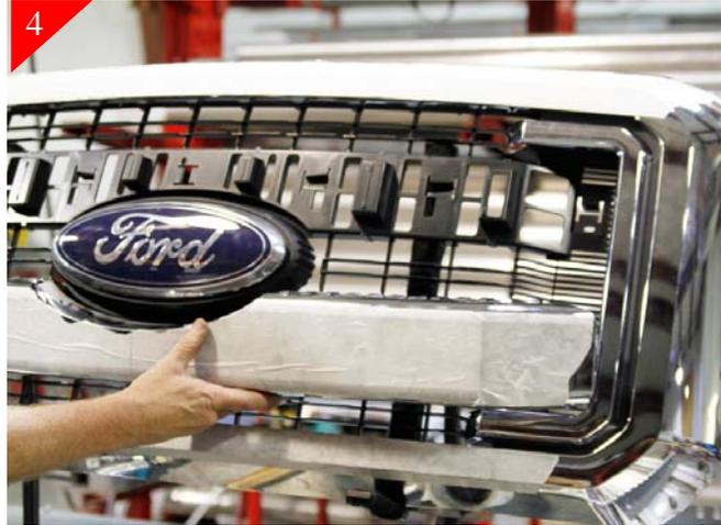
Next you will be removing the (2) large horizontal stock chrome overlays from your vehicle. Do so by releasing the clips from the backside.
