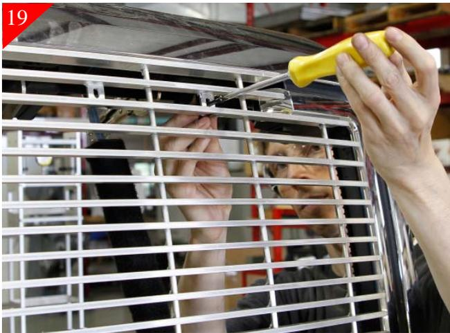
Attach upper brackets to billet grille using the supplied 10-24 x 1" bolts. Again the smaller brackets go to the outside and the larger brackets mount to the inside mounting tabs of billet grille.
