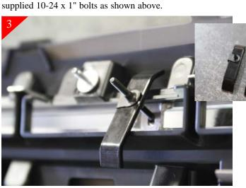
Next you will be attaching the (2) center brackets. Place supplied u-clips on brackets as shown above. Push the supplied 10-24 x 2" bolts through the 2 upper center mounting tabs in billet grille. Next place the brackets and rotate as necessary to catch the backside plastic and then tighten. With all brackets in place check alignment and then tighten all hardware.
