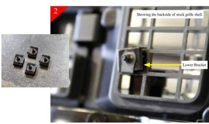
Next place the billet grille into the grille shell and center. Locate the supplied  $10\text{-}24 \times 1 \ 1/4$ " bolts and push through the upper mounting holes in both the upper and lower brackets. Next place the 10-24 u-clips on the square tabs. Then attach the square tabs using the already placed  $10\text{-}24 \times 1 \ 1/4$ " bolts.
