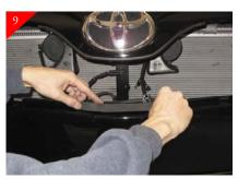
Locate the short piece of the flat molding. Test fit molding in between the two lower brackets trim in necessary. Remove adhesive backing and place as shown
