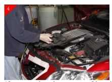
After removing the stock center portion of the stock grille shell. You can replace the plastic core support cover that was removed in Step 2. When replacing the plastic rivets omit the 2 inner rivets or the closest to the front end of vehicle. You will use these mounting holes later in the install.
