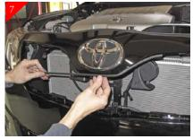
Next you will be attaching the supplied round rubber molding. Start by test fitting the rubber by centering the rubber around logo area of opening. This to get an idea as to where the rubber needs to be. Then peal the adhesive backing off and starting on one end of the rubber attach and slowly work your way around emblem area without pulling or stretching the rubber molding let it naturally follow contour of the logo area.
