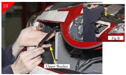
Locate the supplied upper brackets and attach. Do so by sliding the upper bracket under the plastic core support cover. Using the (2) stock mounting holes (See step 4) in core support cover for your attachment point.
