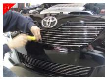
Place billet grille into opening and center. Attach billet grille by using the supplied #10-24 x 5/8" bolts and 10-24 nyloc nuts attach to the already placed upper and lower brackets. Do so by reaching down behind the stock grille shell and tighten.
