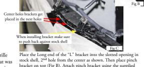
bracket on top (Fig B). Attach pinch bracket using the supplied 10-24 x 5/8" bolts and 10-24 nyloc nuts and tighten. Bracket
