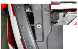
The plastic will hold bracket in place, now place supplied 10-24 fender clip on the bottom side. Followed by placing washers on the top side and attach using the 10-24~x 1" phillips head bolt shown above.
