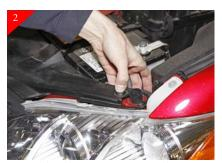
Remove the plastic core support cover by removing the (6) plastic rivets shown above. Remove the rivets by pushing on the center portion of the rivet and remove plastic. This allows you to reach behind the stock grille
