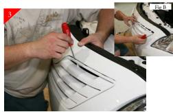
Next you will be removing the center portion of stock shell. Do so by releasing the clips that surround grille shell. Using a regular screwdriver and pushing slightly from the backside will aid in the release of the clips. Take time in releasing clips so as not to scratch painted surface. Continue working around the outside of stock grille shell releasing clips until center is free (Fig B). There are 22 clips total.
