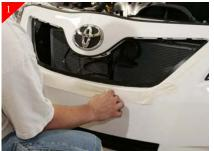
Tape front end of vehicle using masking tape to protect during install.
