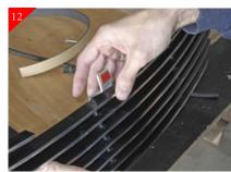
Attach the center bracket that helps align the logo area of stock shell with billet grille. Do so by attaching supplied bracket to mounting tab located in middle of the billet grille. Attach using 10-24 x 5/8" bolt and 10-24 fender clip and tighten as shown. After attaching bracket remove adhesive cover and tape.
