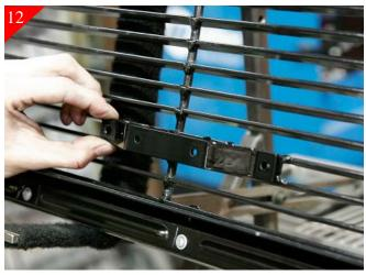
After attaching billet grille you will need to attach the hood release brackets to billet grille. Attach supplied bracket shown above to the mounting tabs in billet grille using the supplied  $10\text{-}24 \times 5/8$ " bolts and 10-24 Nyloc nuts.
