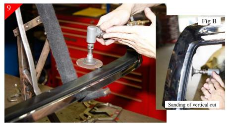
Next sand or grind all cut areas smooth with the shell. (Fig B) Shows the vertical sanding.
