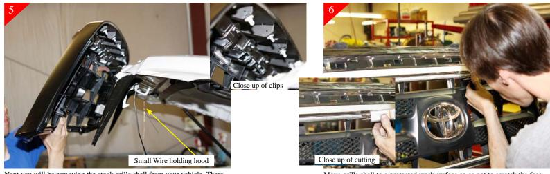
Next you will be removing the stock grille shell from your vehicle. There are plastic clips along the top of the stock grille shell that attach to the hood. Release by pulling out on the grille shell. These clips are for Factory install purposes only. So when removing shell the clips may break.
