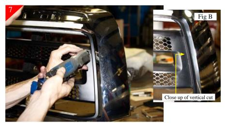
Shown above is cutting of the vertical attachment point. Again leave some material for finish sanding. (See Fig B for after cut photo).
