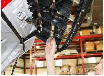
Locate the hood release mechanism and remove the hood release rod shown above but pulling it out of the snap clip holding in place. Rod will pull out with very little tension.
