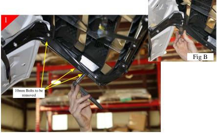
First start by opening the hood on your vehicle. Next there are the (3) 10mm bolts on both the driver and passenger side of the truck that attach the steel brace and the stock grille shell together that need to be removed (Fig A & R)
