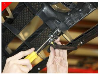
Now you will be removing the hood release lever from the stock grille shell. You will be reattaching the stock lever to the new billet grille in latter steps. Also a small wire or rope can be use to hold the hood at a workable height. Remove before closing hood.
