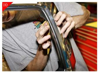
After sanding down smooth with the stock shell, follow up with some finish sanding. We recommend using a 150 grit sand paper.
