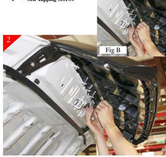
Locate the (6) 10mm bolts shown above that attaches the stock grille shell to the hood of the vehicle and remove (Fig A & B).
