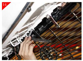
Now you are ready to place the shell back on vehicle. Make sure that you have removed the stock bolts from the top portion of the top brackets. this will leave the top portion of the billet grille loose. Place stock grille shell back on vehicle. Align the plastic clips along the hood line and push in place. Align the top brackets with the tabs in hood as shown above. Attach with the stock 6mm bolts as shown above.
