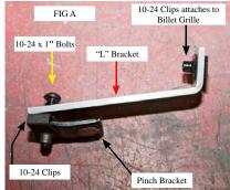
With brackets loosely attached place billet grille into bumper opening and center. Now move the pinch bracket so that
