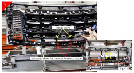
Now for the (2) middle attachment points. Make sure when cutting, to cut as close to the center portion of the grille as you can as shown above. After working your way around and cutting the top (2) middle attachment points just as the lower shown above the center can be removed (Fig A.)
