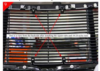
Place billet grille back into opening. Locate the supplied 10-24 x 1" bolts and place thru the middle mounting tabs in billet grille this goes thru the vertical plastic support that you just drilled. Next place the supplied square tabs on the backside of the plastic vertical support onto the just placed bolts now place the supplied 10-24 nyloc nuts to secure.
