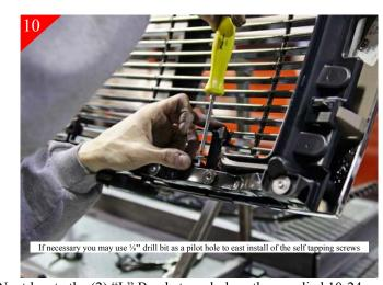
Next locate the (2) "L" Brackets and place the supplied 10-24 u-clips on the long end of the brackets shown above. Attach brackets to the 2 lower outer mounting tabs in billet grille using the supplied  $10-24 \times \frac{9}{8}$ " bolts and attach to the just placed u-clips. Next using the supplied self tapping screws attach the short end of the brackets to the steel framing as shown.
