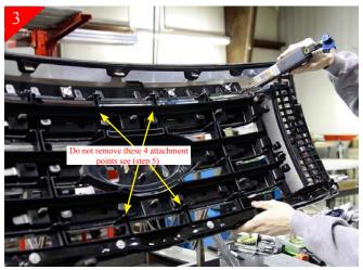
Next you will be removing the center portion of the stock grille shell. Using a air saw cut the vertical attachment points of the grille shell shown above. DO NOT START WITH THE MIDDLE 2 ATTACHMENT POINTS THESE WILL BE ADDRESS IN STEP 5 OF THE INSTALL.
