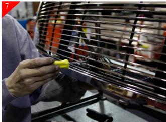
Next turn grille shell over face down, and place the billet grille into the backside of the grille shell opening. Now while holding the billet grille in place flip grille shell and billet grille over face up. Next locate the middle mounting tabs, using a sharpie or scribe mark the mounting hole locations where they meet the middle attachment point left after trimming.
