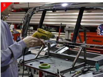
After marking mounting locations remove billet grille from opening. Drill the just marked locations starting with a pilot hole using a ½" drill bit. Next using a ¼" Drill bit re-drill locations.
