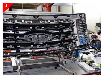
Continuing to work your way around cutting the vertical and horizontal attachment points to remove center portion of the stock grille shell. The center will be removed in the following step.
