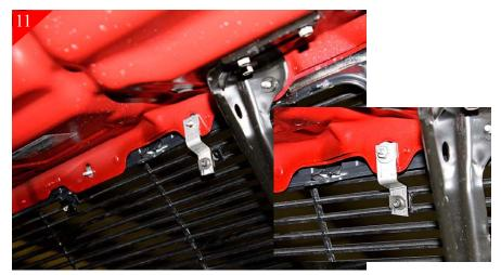
Now locate the remaining brackets and place the supplied 10-24 u-clips on the end of the bracket with a angle bend as shown above. Next place grille shell back on vehicle. Now place the bracket as shown on the mounting stud of the grille shell. Using the supplied 10-24 x 5/8" bolts attach bracket to billet grille. Repeat more remaining side of the billet grille.
