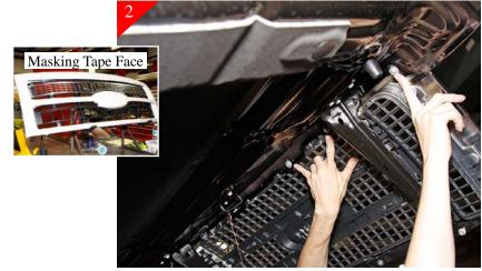
Continuing to remove the stock grille shell. Remove the ( ) 10mm nuts across the top of the stock grille shell holding the top portion of the stock grille shell in place. Remove grille shell and using masking tape, tape the front of the grille shell to protect during the install.
