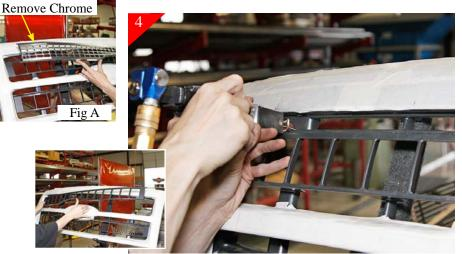
With the chrome facia removed you can now remove the remaining plastic center. Using a cut-off wheel or air saw cut the vertical attachment points, leaving plenty of material to come back and clean up cuts and to do finish cutting and sanding.
