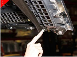
Open hood and remove the () 10mm bolts along the bottom of the stock grille shell holding the stock grille shell in place.
