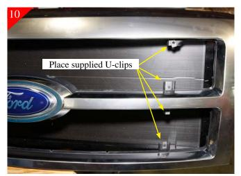
Next place supplied U-clips on all the just drilled locations as shown above. Then insert billet grille back into opening and attach billet grille using the supplied  $10-24 \times 5/8$ " phillips head bolts.
