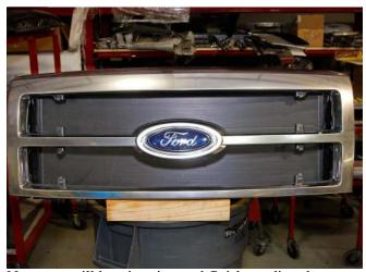
Next you will be trimming and finish sanding the small vertical material left in removing the centers. See image above you will need to LEAVE THE LARGE OUTER VERTICAL PLASTIC, THESE ARE ATTACHMENT POINTS FOR THE BILLET GRILLE.
