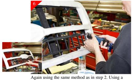
Again using the same method as in step 2. Using a cut-off wheel or air saw cut the vertical attachment points, leaving plenty of material to come back and clean up cuts and to do finish cutting and sanding.
