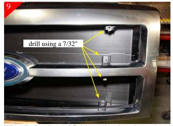
With all trimming and finish sanding done, insert the billet grille into opening and center. Using a sharpie or scribe mark the mounting locations of the tabs where it meets the large plastic verticals. Remove billet grille. Drill all just marked location using a 7/32" drill bit.
