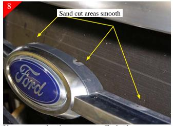
You may use the air-saw or cut-off wheel to remove most of the material. Then come back and finish sand all cut areas smooth.
