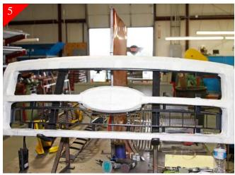
This is with the top portion removed. Now you will cut the bottom portion using the same method as in step 2.
