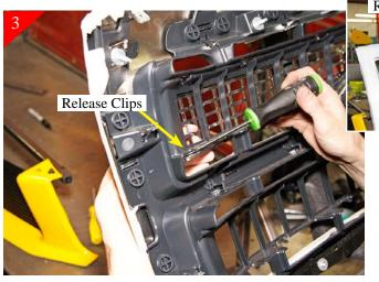
Now you will be separating the chrome Facia from the stock grille shell (Fig A). Do so by releasing the clips on the backside of the stock grille shell. Use a regular screwdriver to lift the plastic clip up to release as shown (Fig B).
