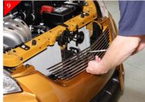
Place billet grille into opening and center. Attach billet grille using the supplied 10-24 x 5/8" bolts. You also may adjust billet grille for center by loosening the bolts and centering and re-tighten bolts.
