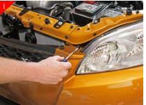
Start by opening the hood and locate the plastic rivets holding the top portion of the stock grille shell in place. Using a regular screwdriver lift up on the center portion and remove rivets.
