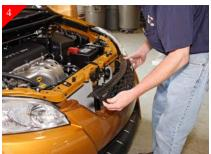
After all clips are released remove the center stock shell.
