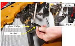
Next you will be attaching the "L" bracket. Place one of the supplied U-clips as shown on the vertical support then attach bracket to the just placed U-clip using the supplied 10-24 x 5/8" phillips head bolts. After attaching place supplied U-clips on other end of the bracket (fig B).
