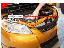
Locate and remove the (2) phillips screws as shown above.
