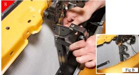
Locate the Long "L" Bracket and attach as shown using the supplied U-clips and 10-24 x 5/8" bolts.
