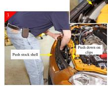
Along the bottom and the sides of the stock grille shell is being held in place by clips (Fig B). You will need to release the clips in order to remove stock shell. Do so by pushing down on the backside of the clips and also pushing back on the stock shell or towards the vehicle.
