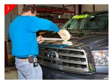
Using masking tape, tape off the hood area just behind the chrome of the stock grille shell. This will protect the hood when removing the grille shell. Also to help hold the hood in a better position for removing grille shell use of a bungee cord or a piece of rope hooked to the hood latch and core
