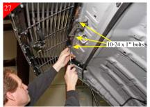
Using the supplied 10-24 x 1" phillips head bolts and #10 fender washers attach as shown above. The bolts will attach to the U-clips that were just placed in the previous (step 25).
