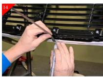
Next you will laying out the holes to be drilled in the stock shell. Do so by using a straight edge to trace the edges of the bracket onto the tape on the stock grille shell as shown above. Then measure ½" from the backside of the grille and mark a center line to be drilled.
