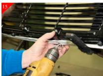
Drill all the just marked hole locations using a 3/16" drill bit.
