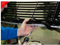
Attach using the supplied 10-24 x 5/8" Phillips head screws. With the bottom secured you will now work on the top brackets.
