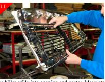
Place billet grille into opening and center. Move steel brace to shell and lay in place and center. Next you will be attaching the steel brace to the 2nd bar from the bottom in billet grille using the brackets along steel brace.
