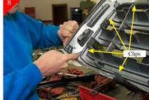
Starting on one end of the grille shell you will be releasing the clips that hold the center section in place. Using a small regular screwdriver to help in releasing clips will be necessary. Once you get several clips released the rest will be much easier.
