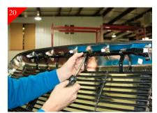
Locate and place the supplied top cross bar as shown. Then attach brackets to the top bar using the supplied U-clips and  $10\text{-}24 \times 5/8$ " philips head screws.
