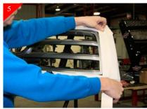
Move stock grille shell to protective surface. Using masking tape, tape the face of the grille shell to protect during install of billet grille. Flip stock shell
