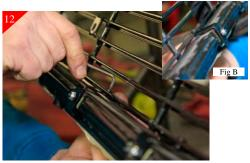
With the bracket under the bar of the billet grille attach using the supplied  $10-24 \times 1/2$  soc head bolt and 10-24 low profile nyloc nut. When tightening use of a ball end Allen wrench or a shortie as shown above will be necessary.
