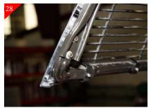
Next you will be attaching the bottom steel brace to the vertical steel brace coming off the hood. Attach using the supplied 1/4-20 x 3/4" soc head bolt and 1/4" washer followed by washer and 1/4-20 Nyloc nuts. Washers go on both the head side and backside. Use of an open end wrench will be necessary in securing. Install is complete.
