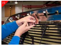
Attach brackets to billet grille using the supplied  $10-24 \times \frac{1}{2}$ " soc head bolts and 10-24 low profile nyloc nuts. See previous step for orientation of brackets.
