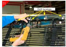
Locate and drill the (5) mounting holes as shown using a 3/16" drill bit. Make sure and check alignment of billet grille before drilling. Be sure the billet grille is flush with stock grille shell. Using caution when drilling so as not to go thru grille shell.
