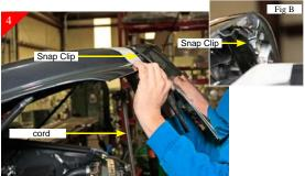
Next you will release the snap clips from across the top of the stock grille shell. Starting at one end, work from the corner to the other end releasing clips. Once you get 1 or 2 clips released the others will come out easier. The use of a door panel removal tool to help pry clips loose will be necessary. These fasteners are very secure and can be tight. (Fig B) shows what the clips look like. Also note that the clips can be located in between the bolts removed in (step 2).
