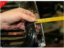
Next you will be centering the billet grille and steel brace to the opening. Using a measuring tape, measure both sides and center as shown above. Should be approximately 1" from the side of the stock shell.
