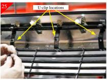
Place the supplied U-clips on the center hole of the (4) vertical upper brackets shown above.
