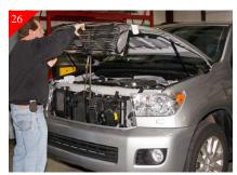
Place the grille shell back on the vehicle. Align the snap clip across the top of the shell with the hood and snap in place. A slight bump with the palm of your hand where the clips are will seat in place.
