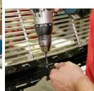
Drill all the just marked hole locations using a 17/64" drill bit.
