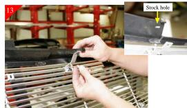
Loosely attach (2) upper brackets to the 2 inner mounting tabs in billet grille using the supplied  $1/4-20 \times 1''$  bolts and 1/4-20 Nyloc nuts. Now attach brackets to top of shell using the stock hole as shown above (Fig B), and also using the stock bolts. This will help hold billet grille in place while marking and drilling remaining mounting locations.
