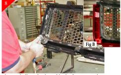
Continue grinding plastic weld tabs from around center portion (only) of stock shell.
