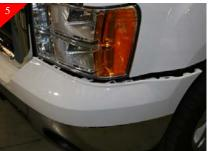
Starting at the corner of the bumper pull out on the painted portion of the bumper grille to release the clips holding in place.
