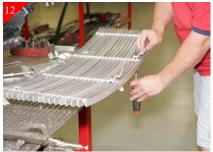
loosely attach the (2) bottom brackets using the supplied  $1/4-20 \times 1$ " Bolt and 1/4-20 Nyloc nuts shown above.
