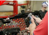
Lay shell on protective work surface. Tape the chrome portion of the stock grille shell using masking tape to protect during install. Now turn grille shell over face down. Using a grinding wheel grind the plastic weld tabs from across the top of the grille shell as shown above.
