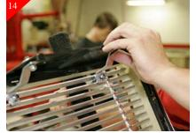
Now loosely attach the remaining (2) upper brackets to billet grille using the supplied  $1/4-20 \times 1^{\circ}$  bolts &  $1/4^{\circ}$  Flat washers and 1/4-20 Nyloc nuts. The washer go on the head side of the bolt or on top of plastic.
