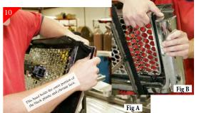
With all weld tabs ground remove center portion of stock grille shell. With one hand hold the outer portion of the shell (Fig A). The other on top with fingers thru holes of the face of shell and pull or leverage up with thumb on the outer portion of shell (Fig B).
