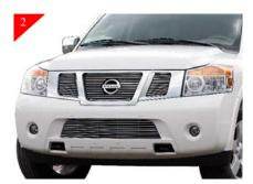
Place billet grille into opening and center. Place supplied 10-24 x 2" bolts thru mounting tabs in billet grille. Attach brackets on the backside of the stock shell without over tightening.
