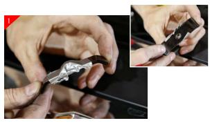
Start by locating the supplied brackets and 10-24" nyloc nuts. To make the installation of the brackets easier, tape the nut on the backside of the bracket as shown. You can remove the tape after you get the bolt started.
