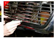
Place billet grille into opening and center. Making sure to push billet grille back into opening so that the billet grille seats or rests against the raised portions of the upper and lower opening. Now using a 90° scribe mark the locations of all the mounting holes (8) total. Remove billet grille.
