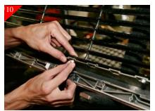
Place billet grille back into opening and center. Attach billet grille using the supplied 10/32 x 1/2" bolts and 10/32 nyloc nuts.
