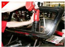
Drill all just marked locations using a 7/32" drill bit.
