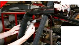
Using a grinder or sanding block sand the cut areas smooth for driver and passenger side of stock shell. Now sand the top and bottom of the stock shell just to clean up cut areas. Do not sand flush! These raised areas are needed to register billet grille into opening and will not be seen after billet grille is installed.
