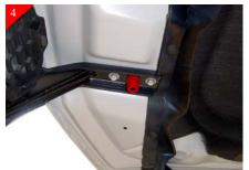
Remove the two rubber stops on the brackets and **SAVE** them. They will be reinstalled. Move to a protective work surface.
