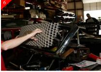
After cutting remove center portion of stock grille shell.
