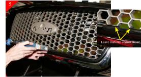
Using a air saw or other cutting devise remove center portion of the stock grille shell leaving material shown in (Fig B) along the top and bottom of grille shell.
