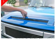
Next you will be preparing for drilling the center mounting hole. Do so by pushing slightly down on the center portion of the insert as shown. This will align the insert properly with hood opening. You will need to hold the insert in this position during the first drilling process. Using 1/16" drill bit drill the center mounting hole. Now remove the CNC machined grille from opening and finish drilling the center mounting hole using the larger 3/8" drill bit.
