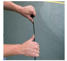
Your Insert needs to follow the contour of your hood. It maybe necessary to form the insert slightly by bending as shown above due to shipping. Be very careful around the mounting holes during this process as it my bend to much and or crack the mounting hole.
