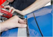
After centering check alignment of insert. Starting with 1/16" drill bit and then moving to a larger 3/8" drill bit as shown above drill ONLY the outer (2) mounting holes. After drilling attach using the supplied 10-32 well nuts and 10-32 x 5/8" bolts. Place well nuts into just drilled locations and seat against the hood opening then attach using the 10-32 x 5/8" bolts.
