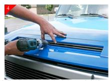
After drilling the center mounting hole. Attach CNC machined grille using the supplied 10-32 x 5/8" bolts and 10-32 well nuts. Install is complete
