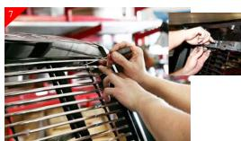
Repeat steps 5 and 6 for the remaining mounting hole locations. After all mounting holes have been drilled. Secure the billet grille by using the supplied 10-32 x 1/2" SS bolts and 10-32 nyloc nuts.
