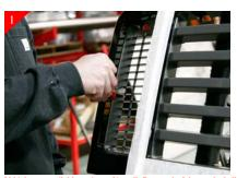
Vehicle not available at time of install. Removal of the stock shell is not necessary but will facilitate the install. Move the grille shell to a protective work surface. Start with the 2 vertical openings of the stock shell as shown above. Using a pair of flush cut cutters cut all the vertical and horizontal attachment points flush with the shell. Remove plastic and discard.
