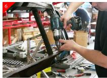
Drill just marked location using a 7/32" drill bit. Place billet grille back into opening and using one of the bolts place into mounting hole without using nyloc nut. This is just to make sure the mounting holes line up and billet grille doesn't move during marking of remaining mounting holes.
