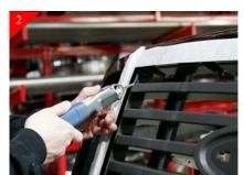
Now you will be removing the center portion of the stock shell follow steps 2 thru 4 for removal. Do so by using an air saw or other cutting device, cut along all vertical and horizontal attachment points close to shell.
