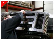
Locate and remove the (7) Plastic Phillips head screw clips that hold stock grille shell in place. They are located along top of stock grille shell. To aid in removing squeeze the backside of the clip to keep the screw threads engaged.
