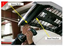
Open hood and locate and remove the (2) 8mm bolts (1) per side of stock shell that attach stock grille shell to steel brackets shown above.
