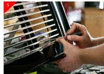
Using a 90° scribe mark the hole locations for (1) of the mounting holes and remove the billet grille.
