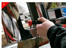
Drill just marked mounting hole location using a 7/32" drill bit. Place billet grille into opening and using (1) of the supplied bolts place into mounting hole without using the nyloc nut. This is just to make sure the mounting holes line up and billet grille doesn't move during marking of holes. Now using the 90° scribe mark the other mounting hole location and remove billet grille. Repeat drilling process.
