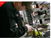
After both mounting hole locations have been drilled. Attach billet grille using the supplied 10-32 x 1/2" and 10-32 nyloc nuts.
