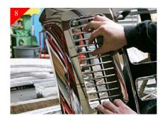
Now for the 2 vertical openings place billet grille into opening and center. Make sure to push billet grille into opening and seat against the grey plastic in opening. Using a 90° scribe mark the hole locations for (1) of the mounting holes and remove the billet grille.
