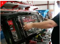
Place billet grille into opening and center. Check for alignment.
