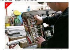
Starting with the wing portion place billet grille into opening and center. Make sure to push billet grille into opening and seat against the grey plastic in opening. Using a 90° scribe mark the hole locations for (1) of the mounting holes and remove the billet grille.
