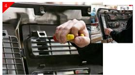
Move the grille shell to a protective work surface. Turn shell over face down. Then using cutters cut all the vertical and horizontal attachment points. (Fig B) shows the removal of the plastic inner. Repeat for all openings.
