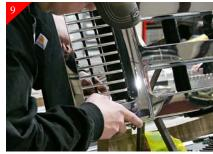
Attach billet grille using the supplied  $10-32 \times 1/2$ " and 10-32 nyloc nuts. Place bolts into mounting holes and secure with nyloc nuts.
