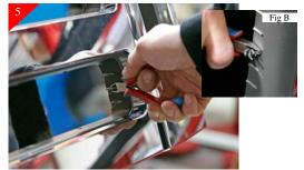
After all plastic centers have been removed clean up cut areas by using a pair of flush cut cutters and trim flush with stock shell as shown above. Flush cut cutters will allow you to cut as close as possible to stock shell without the need of sanding. Close up of trimming (Fig B).
