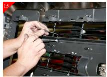
Place Top billet grille in place and center and attach using the supplied 10-32 x 1/2" and 10-32 nyloc nuts as shown above.
