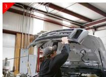
The stock grille shell is being held in place by snap clips across the top of the shell that clip into hood. Release these clips by supporting with one hand and with the other using a bumping motion or push towards the vehicle to release.
