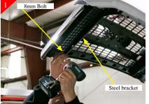
Open hood and locate and remove the (2) 8mm bolts (1) per side of stock shell that attach stock grille shell to steel brackets shown above.
