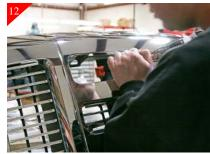
Repeat installation process for all openings with the exception of the TOP BILLET GRILLE. Mark and drill as in previous steps without attaching the billet grille. You will attach the billet grille after the stock grille shell has been placed back on the vehicle. The reasoning behind this is that you would not be able to reach the (7) plastic phillips head clips that you removed in step 2.
