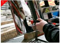
Drill just marked location using a 7/32" drill bit. Place billet grille into opening and using (1) of the supplied bolts place into mounting hole without attaching nut. This is just to make sure the mounting holes line up and billet grille doesn't move during marking of holes. Now using the 90° scribe mark the other mounting hole location and remove billet grille.
