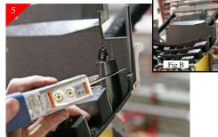
Lay stock grille shell face down on a protected work surface. Locate the (2) stock mounting clips shown above. (Fig B) shows mounting clip removed.
