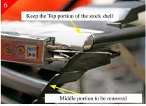
Now you will be removing the top portion of the stock shell from the middle portion. Using an air saw or other cutting devise remove starting at one corner as shown. See next step for more cutting instructions.
