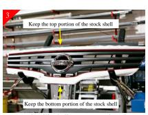
Next move stock grille shell to a protected work surface. Next you will removing the center portion of stock shell. You will need to keep the top and bottom portion of the stock shell for the installation of billet grille. See next step for cutting instructions.
