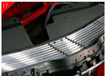
Following the same procedure as in step 16, align the billet grille with the top portion of the stock shell. Using vise grips to clamp in place. Using the supplied  $10-32 \times 5/8$ " bolts, place bolts in just drilled locations and secure with the supplied 10-32 nyloc nuts.
