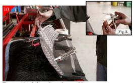
Tape a pair of vice grips using masking tape to protect during the clamping process (Fig A). Align the billet grille with the top portion of the stock shell. Then use the vice grips to clamp one end and then align and clamp the other end in place. Adjust as necessary to get the correct alignment.
