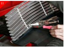
After aligning using a 90° scribe mark the mounting locations where it meet the stock shell as shown above. After marking remove billet grille.
