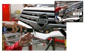
Starting with the bottom cut the vertical attachment points using an air saw or other cutting devise as shown above. Make sure and leave material so that you can come back and do finish sanding. (Fig B) Shows removal of bottom portion of the stock grille shell after cutting.
