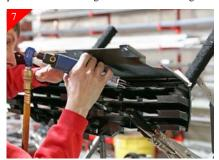
Turn stock shell over face down and cut all the vertical attachment points using an air saw or other cutting devise as shown above. Make sure and leave material so you can come back and do finish sanding.
