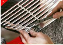
Align billet grille with the bottom portion of stock shell. Again using a pair of taped vice grips clamp in place. Using the supplied  $10-32 \times 5/8$ " bolts, place bolts in just drilled locations and secure with the supplied 10-32 nyloc nuts.
