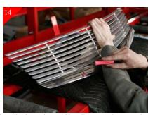
After aligning using a 90° scribe mark the mounting locations where it meet the stock shell as shown above. After marking remove billet grille.
