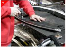
Using a air sander or sanding block, sand all cut areas smooth with shell for both the top and bottom portions of stock shell.
