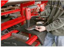
Drill the just marked hole locations using a 3/16" drill bit as shown above.
