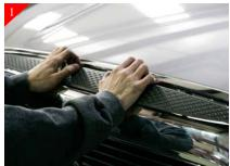
Remove the plastic rock guard from top of stock shell. Do so by unclipping at one end and working to the other.
