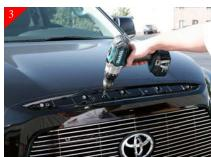
Remove machined grille and drill the just marked hole locations. Drill using a 3/16" drill bit as a pilot hole then move to a 3/8" drill bit and drill again as shown. Repeat process for remaining attachment holes.
