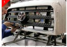
Using a air saw or other cutting devise. Remove the center portion of the stock grille shell by cutting all the horizontal and vertical attachment points. Make sure and leave material for finish sanding. See step 6 for cutting the vertical attachment point.
