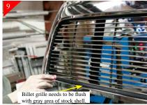
Place billet grille into opening and center. Make sure billet grille is flush top and bottom before marking. Using the billet grille as a guide, mark the hole location using a sharpie or scribe (4) on top (4) on bottom. After marking remove billet grille and Drill just marked location using a 7/32"
