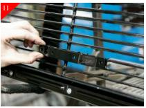
After attaching billet grille you will need to attach the hood release brackets to billet grille. Attach supplied bracket shown above to the mounting tabs in billet grille using the supplied 1/4-20 x 5/8" bolts and 1/4-20 Nyloc nuts.
