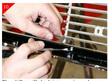
Place billet grille back into opening and center. Attach billet grille using the supplied  $10\text{--}32 \times 1/2$ " bolts and the 10--32 nyloc nuts.
