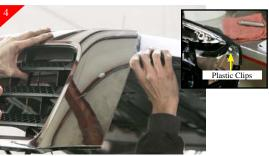
Next there are (2) plastic snap in clips one per side of stock grille shell. You need to pull out on the upper corners of the stock shell to break these clips. These clips serve only as a manufacturing aid. They don't have any structure of supporting functions. Also they are difficult to see but they are there. Grille shell will be free at this
