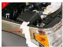
Tape as shown above to protect during the removal of stock shell.
