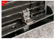
The bottom brackets attach using the supplied #8 x 5/8" Phillips head screws and U-clips as shown above.
