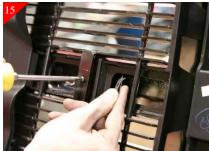
With all holes drilled. Place the billet grille back into opening and attach brackets to billet grille just as before. Now you will be attaching the billet grille to the stock shell. Starting with the center attachment, place supplied U-clip on the backside and attach using the supplied #8 x 1" Phillips head screw as shown.
