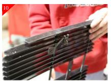
Note: Photo was taken while billet grille was not in stock shell to better show the attached bracket. Place supplied U-clip on Upper bracket as shown above. Then attach the bracket to billet grille using the supplied #8 x 5/8" Phillps head screw
