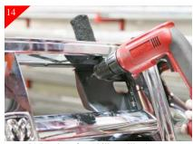
Remove the brackets from billet grille then remove billet grille from opening. Then using a 3/16" drill bit, drill all the just mark locations. When drilling holes for the center attachment be careful to not drill thru the chrome portion of the stock shell.
