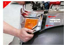
Starting on the drivers side of the vehicle. Unsnap the stock shell, when you get in started as shown above, place your hand fairly low on the shell and pull straight out on the stock shell to release from
