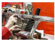
Mark The hole location for the Upper bracket using a scribe as shown.
