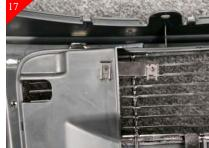
To Attach the Upper bracket locate the hole you drilled and place a supplied U-clip on the backside of plastic and attach by screwing to the U-clip as shown above. Install is complete. Center stock shell on vehicle and snap shell back in place and remember to attach all headlight connections. (Ref. steps 1-6).
