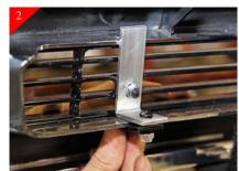
Start by loosely attaching the supplied "L" bracket to billet grille using the supplied 10-24 x 5/8" bolts and the 10-24 nyloc nuts as shown above. Then attach the supplied smaller pinch bracket to already placed "L" bracket using the 10-24 x 5/8" bolts and 10-24 nyloc nuts as shown above.
