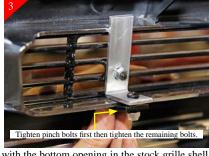
Starting with the bottom opening in the stock grille shell. Place the billet grille into opening and center. Reaching thru the upper opening rotate the brackets around so that it catches the lip of the opening. Tighten the smaller pinch brackets as shown, then tighten the bolts that secure the billet grille to the brackets.
