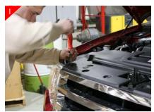
Open hood and remove the plastic Phillips head screws that hold the plastic core support cover as shown above.
