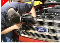
For The top billet grille, reach thru from the top and rotate the brackets around, again following the same procedures as in steps 2 & 3. Replace the plastic cover that was removed in step 1. Install is complete.
