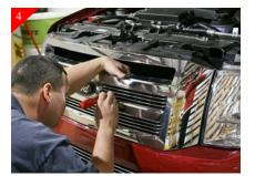
Using The same procedure as in step 2-3, install billet grilles into the next openings up from the bottom.
