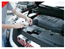
Start by removing the plastic core support cover. Do so by removing the plastic push pull style rivets as shown above. Using a small regular screwdriver lift on the center portion of the rivet to release. Remove the core support cover.
