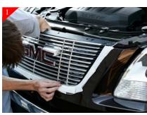
Place billet grille into opening and center. Attach billet grille by using the supplied 10-24 x 1" bolt and 10-24 nyloc nut and square tab. Place bolt thru mounting tabs in billet grille. Then reaching down behind stock grille shell place the square tab on the just placed bolt followed by the nyloc 10-24 nut. (See Diagram)
