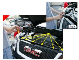
With core support cover removed, remove the (6) phillips head screws holding top portion of the stock grille shell in place. Also remove (2) more of the plastic push pull style rivets located just outside of the chrome on stock shell on driver and passenger side of shell (Fig B). This allow you to reach behind the stock grille shell.
