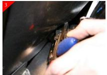
Reaching between the stock grille shell and the radiator locate the (4) clips along bottom of stock shell shown above and using pliers squeeze the clip together to release as shown.
