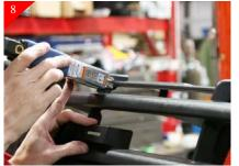
Using a air saw or other cutting devise. You will be removing the center portion of the stock shell. Cut all horizontal and vertical attachment points flush with shell. Making sure to leave enough material to do finish sanding. See (step 9) for more cutting images.
