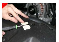
Remove the (4) plastic push pull rivets from along top of core support.
