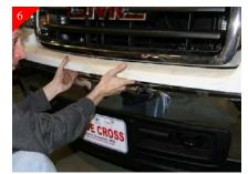
Moving out to the center of the painted bumper area again pull out to release the clips. Now at this point you will be able to separate the stock chrome shell from the bumper. Grille shell will be free at this point.
