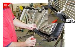
After drilling attach brackets using the supplied 1/4-20 x 1" bolts and 1/4-20 Nyloc nuts. Make sure the bottom brackets are butted against the black plastic (Fig B).
