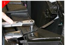
Remove the (4) 10mm nuts from top of stock grille shell.
