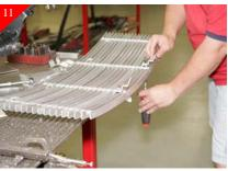
loosely attach the (2) bottom brackets using the supplied  $1/4-20 \times 1''$  Bolt and 1/4-20 Nyloc nuts shown above.
