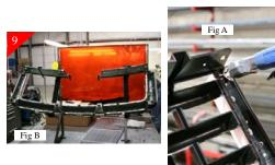
(Fig A.) shows cutting of the horizontal attachment points. (Fig B.) shows after cutting all attachment points and center removed.
