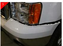
Starting at the corner of the bumper pull out on the painted portion of the bumper grille to release the clips holding in place.
