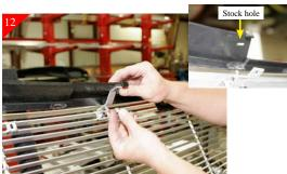
Loosely attach (2) upper brackets to the 2 inner mounting tabs in billet grille using the supplied 1/4-20 x 1" bolts and 1/4-20 Nyloc nuts. Now attach brackets to top of shell using the stock hole as shown above (Fig B), and also using the stock bolts. This will help hold billet grille in place while marking and drilling remaining mounting locations.
