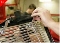
Now loosely attach the remaining (2) upper brackets to billet grille using the supplied 1/4-20 x 1" bolts & 1/4" Flat washers and 1/4-20 Nyloc nuts. The washer go on the head side of the bolt or on top of plastic.
