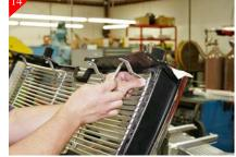
Using a scribe mark the mounting location where is meets the top of the shell as shown above.
