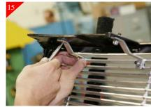
Repeat for other side--Using a scribe mark the mounting location where is meets the top of the shell as shown above.
