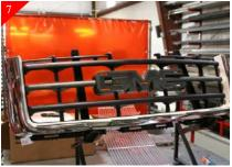
Move stock grille shell to a protected work surface. Using masking tape, tape the chrome portions of stock grille shell to protect during install.
