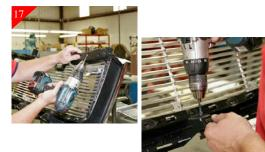
Drill all the just marked hole locations using a 17/64" drill bit.
