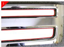
Pictured above is after cutting, sanding cut areas is optional. Do not remove material shown in "RED" in (Step 2).
