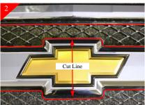
Remove stock grille from the vehicle by removing plastic push pull rivets from across core support. The grille shell is held in place with snap clips. Locate the 4 along bottom of shell and 2 located on both sides of the emblem. Then cover painted and chrome finishes to protect from damage during installation.
