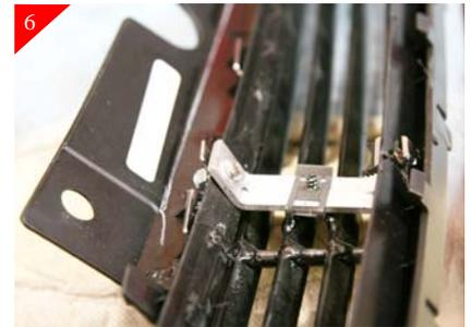
Place supplied u-clips on middle hole of the supplied brackets. Place billet grille into opening and center. Attach brackets to billet grille using the supplied #8 x 5/8" Phillips head screws. Check fitment and mark the hole locations of the brackets where it meets the stock shell. Remove billet grille from opeing, then using a 3/16" drill bit , drill the just marked locations. Shown above is with the bracket completely attached.
