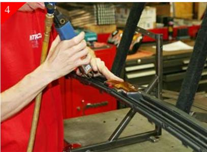
Using a air saw or cut off wheel, remove the center portion of the black plastic backing, leaving some material so that you can do finish sanding, see step 5 for further explanation.
