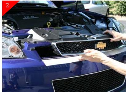
With rivets removed unsnap the grille shell from vehicle as shown above.
