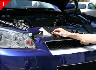
Start with placing protective masking tape on vehicle to protect during install. Locate and remove the plastic rivets across top of core support as shown above.
