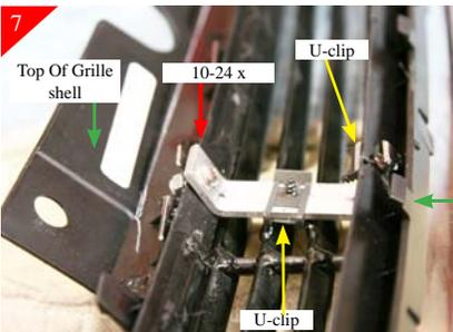
After drilling holes, remove the brackets from billet grille. Place a supplied U-clip on the brackets as shown above. Then attach to U-clip using the supplied #8 x 5/8" Phillips head screws. Place a supplied 1/4-20 x 1/2" thru hole in bracket and attach using the 1/4-20 Nyloc safety nut as shown above.
