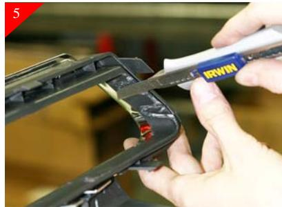
With center poriton removed, you will need to clean up all the cut areas. Using a sanding block to smooth out, but you might find it easier to use a utility knife in cleaning up these areas.
