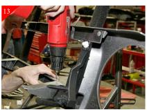
Drill all marked locations using a 3/16" drill bit as shown above.
