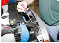
Next locate (2) clips shown above and release using a regular screwdriver to aid in the release. With the top clips released now locate the (3) clips along bottom of stock grille shell and release using the same method as the top.
