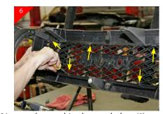
Using a regular screwdriver locate and release (8) plastic clips holding center portion of stock grille shell in place.
