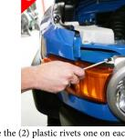
Locate the (2) plastic rivets one on each end of the stock shell shown above and remove.
