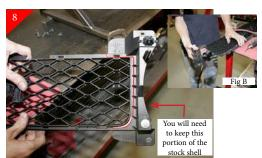
Using a sharpie mark a cut line as shown above in red. Repeat for other side of stock shell. Using a cut-off wheel or other cutting device cut along marked line again repeat for other side of shell. (Fig B) shows after cutting.
