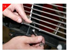
After drilling place billet grille back into opening and center. Attach billet grille using the supplied  $10\text{-}32 \text{ x } \frac{1}{2}$  bolts and 10-32 Nyloc nuts. Place supplied bolts thru mounting tabs in billet grille and thru the just drilled locations and attach using the nuts on the underside of the stock shell as shown.
