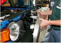
Stock shell will be free at this point. Remove and lay stock shell face down on a protected work surface.
