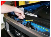
Remove (2) 10mm bolts that hold stock grille shell in place.
