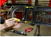
Locate and remove the (6) phillips head screws located on backside of stock grille shell as shown above.
