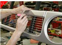
After aligning billet grille mark the (6) mounting locations using a 90° scribe as shown above. After marking remove billet grille from opening.
