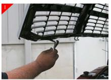
Start with removing the (12) 8mm. Bolts from the backside of the stock grille shell as shown. Grille shell will be free at this point. With shell removed tape the face of the grille shell to protect during install.
