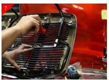
Place Billet grille back into opening and attach billet grille to the just placed u-clips using the supplied  $\#10 \ge 1 \ 1/2$ " Phil pan head screws.
