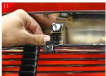
Place supplied U-clips on the just drilled hole locations. Now attach bracket to stock shell using supplied #8 x 5/8" Phil pan head screws.
