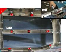
After plastic inserts are removed you will need to grind off the tabs shown in RED above (Fig A). Using a grinder or cut-off wheel, hacksaw ect.. Grind or cut then sand smooth as shown (Fig B).
