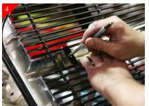
Place billet grille into opening and center. Next using a scribe mark the hole locations where the mounting bracket meets the stock grille shell as shown above. Repeat for the other center brackets.
