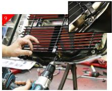
After attaching brackets mark the location of the holes using a scribe. Then using a 3/16" drill bit drill the just marked locations. After drilling place a supplied U-clip on the just drilled location. Then attach bracket using supplied #8 x 5/8" Phil pan head screws. (Fig B.) shows the final attachment of the bottom bracket.
