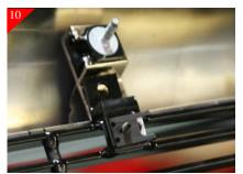
Attach Top brackets to billet grille using the supplied U-clips and  $\#8 \ge 5/8$ " Phil pan head screws as shown above. Using a scribe mark the hole locations where it meet the stock shell. Drill just marked holes using a 3/16" drill bit.
