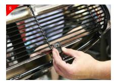
Attach the supplied Bottom brackets to the billet grille using the supplied U-clips and #8 x 5/8" Phil Pan head screws as shown above.
