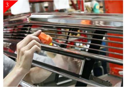
Place top portion of billet grille into opening and align. **NOTE: The difference in the (2) billet grilles is that the TOP bar in the bottom portion of billet grille is angled.** Attach billet grille to the already placed brackets using #8 x 5/8" Phil pan head screws. Now go back and tighten up all the brackets.
