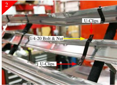
Attach the (2) middle brackets as shown using the supplied 1/4-20 x 3/4" bolts and 1/4-20 nyloc nuts. Again do not fully tighten at this point. Place supplied U-clips on both ends of the brackets.
