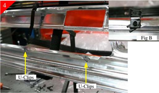
Place the (4) supplied U-clips in stock mounting holes along bottom of shell as shown above. If the mounting tabs get bent it maybe necessary to bend back and or flatten, this can be done using your hands. Now attach supplied bottom brackets to the just placed U-clips using the supplied #8 x 5/8" Phil pan head screws as shown above (Fig B). Place supplied U-clips on other end of brackets.
