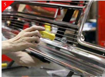
Place bottom portion of billet grille into opening and align. Attach billet grille to the already placed brackets using the supplied #8 x 5/8" Phil pan head screws as shown above.
