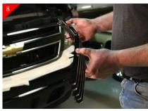
Place the supplied bolts in bottom billet grille as shown above. Then place billet grille into opening and center.
