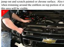
Remove (6) 10mm. bolt from along core support area. This will alow you to reach behind the stock shell.
