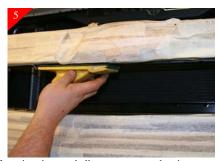
After trimming sand all cut areas smooth using a sanding block.
