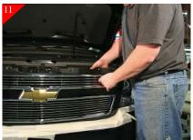
Place the top billet grille in place and center. Then attach using the same method of attachment as the bottom billet grille (steps 8 thru 10). After tightening re-install the (6) 10mm. bolts that were removed in step 7.
