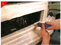
Using a hack saw go back and trim all the cut areas or if using a air saw as shown above, take care in trimming as the saw can jump out and scratch painted or chrome surface. Also take care when trimming around the emblem on top portion of stock shell as this great will be vicible.
