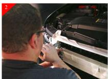
Remove the "Egg Crate" section by using a pair of dykes to snip out as shown above. You are just removing the bulk of the "egg crate" section as much as you can.
