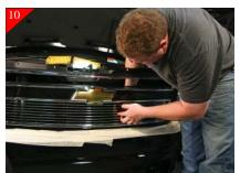
Place the supplied brackets on the backside of grille shell and tighten using the supplied 1/4-20 nyloc nut. It's recommended to start all the nuts before tightening.
