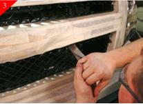
Repeat the cutting process for the bottom portion of the stock grille shell as shown above.
