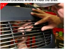
With the bottom brackets attached place the billet grille back into opening and center. Place the spacer between the billet grille and the shell (Ref. step 11), then attach using the supplied  $1/4-20 \times 3/4^{\circ}$  Soc head bolts and 1/4-20 nuts
