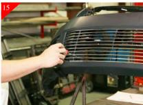
Attach the bottom using the supplied #8 x 5/8" Phillips head screws as shown above.
