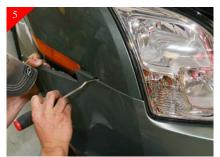
Starting on either side of the vehicle. Using a pry tool or screwdriver. Release the clips holding front end in place. Push pry tool in and lift up on the clip to release.
