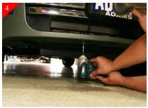
Using a 7mm socket remove the (10) bolts from under front end as shown above.
