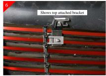
After drilling attach using the supplied #8 x 5/8" Phillips head screws.
