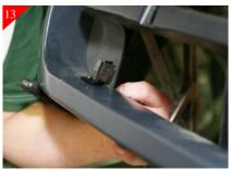
Remove the bottom brackets from billet grille and attach them to the shell. Using the supplied  $1/4-20 \times 3/4^{\circ}$  Soc head bolts and 1/4-20 nuts as shown above.
