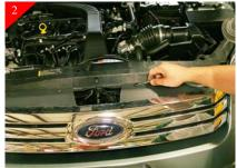
Remove plastic rivets across top of core support. A small regular screwdriver will aid in removing.
