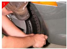
Now Locate (3) per side in wheel wells plastic rivets & remove.
