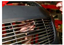
Next place the supplied spacer between the billet grille and the shell, then place the supplied 1/4-20 x 3/4 soc head bolt into hole. This will hold the spacer in place while marking the bottom brackets for drilling. Now mark the hole locations for the bottom brackets where it meet the shell.
