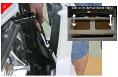
With center section removed, you will need to shave off the raised section of the BACKSIDE of the bottom (2) tabs. Lean the grille shell forward and then using a utility knife shave off the raised sections as shown above.
