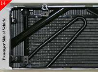
Attach the bottom bracket as shown long end of the bracket to the truck. Attach the top bracket as
