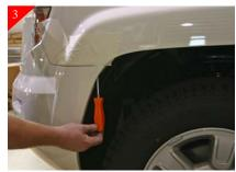
Remove (1) Phillips head bolt per side of vehicle as shown above.
