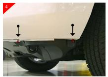
Then remove the (2) 10mm bolts per side of vehicle as shown above. (Bolts are shown in RED.)
