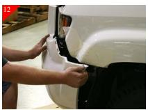
After paint has dried remove cardboard and snap the front end back to vehicle and attach using the 10mm bolts.
