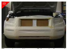
Then using masking off the entire front end. **NOTE: TAKE TIME** to ensure that no over spray get on vehicle. You may want to use 4" wide tape to make taping faster and then use 3/4" to get into the corners.
