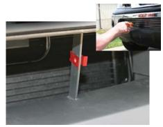
Next place the u-clip on plastic fin as shown above. The u-clip must go on from the backside. Then attach the brackets to the u-clips. Place billet grille back into opeing a center then attach billet grille to the bracakets using #8 x 5/8" Phil Pan head screw.
