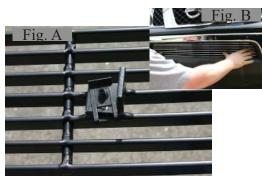
Start by attaching U-clip to bracket. U-clip attached on the slotted hole side of bracket (Fig. A). The round hold attaches to truck. Then attach bracket to Billet Grille using #8 x 5/8" Phil Pan Head screw. Next place billet bumper grille into opening and center (Fig B).
