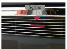
Using a Scribe mark the locations of the Brackets against the plastic fins as shown above. After marking remove the grille and remove the brackets from the billet grille. The drill a 3/16" hole in each of the marked locations.
