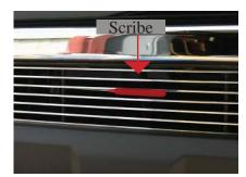
Using a Scribe mark the locations of the Brackets against the plastic fins as shown above. After marking remove the grille and remove the brackets from the billet grille. The drill a 3/16" hole in each of the marked locations.
