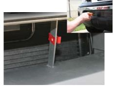
Next place the u-clip on plastic fin as shown above. The u-clip must go on from the backside. Then attach the brackets to the u-clips. Place billet grille back into opeing a center then attach billet grille to the brackets using  $\#8 \times 5/8$ " Phil Pan head screw.
