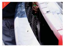
Next pull the stock shell slightly forward, and reaching behind the stock shell release the (5) clips at the bottom of the stock grille shell. If needed use a flat blade screwdriver to aid in releasing the clips as shown above.
