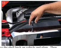
Place the shell back on vehicle and align. Then replace the stock 7/32" bolts that attach across the top of shell.
