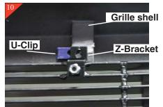
Loosely attach the (Z) shaped brackets at all other locations. Using supplied 1/4-20 x 5/8" Bolts and Nuts. Next place "U" Clips on stock shell and align with bracket as shown. Next tighten all bolts.
