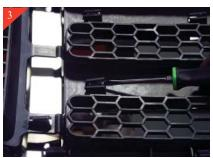
Tape off the face of the stock grille shell using masking tape. This will protect grille shell during install. Next lay shell face down on a protective surface. Then using a flat blade screwdriver pry out to release all clips holding center sections of stock grille shell as shown above
