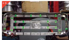
(Fig. 4B) All the tabs marked in GREEN need to be removed
