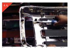
Next using a cut-off wheel or a hack saw it will be necessary to remove some of the tabs (Fig 4A). The next step (Fig. 4B) shows the tabs that need to be removed.
