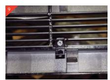
Loosely attach the (L) shaped brackets to the bottom of billet grille, with the short side of bracket attaching to billet grille as shown above.
