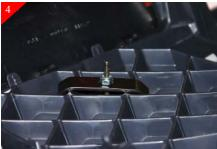
Insert the billet grille and center into the openings. Use the supplied hardware to attach the billet grille to the factory grille shell. Tighten all bolts, being careful not to over tighten. As shown above.
