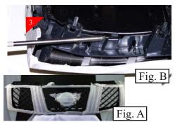
Place masking tape on all of the painted and or chrome surfaces to protect the grille from scratches during install (Fig A). Next remove the plastic shroud covers on the outer left & right side of the stock grille shell. You may have to use a flat blade screwdriver to release. As shown above (Fig B).
