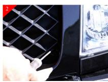
On the lower outsides of the grille shell there are (2) quarter turn screws that can be reached by going thru the lower opening on the side of the grille as shown above.
