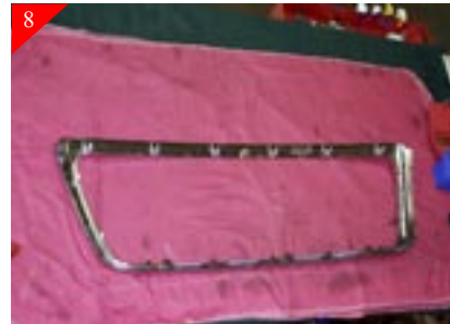
With the tabs released, the grille shell can now be removed from the honeycomb grille. Here is a picture of the frame without the honeycomb grille.
