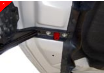
Remove the two rubber stops on the brackets and SAVE them. They will be reinstalled.
