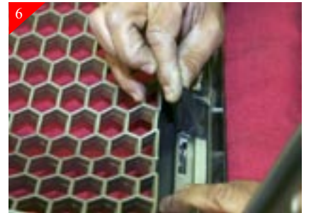
Now separate the outer shell from the honeycomb factory grille, but first you need to remove the fiber tape covering the clips.
