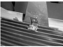
**STEP 6** Now place the billet grille into the back of grille shell. Center the grille in the opening. Place the Short L-Brackets on the tabs at the Bottom of the grille and mark location of the the slots & drill a 1/8" hole. Attach using supplied screws.
