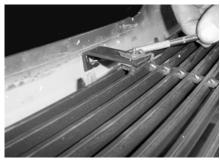
**STEP 7** Place the Long L-Brackets on the top of the grille as shown and mark locations of slots in brackets & drill a 1/8" hole. Attach brackets using supplied hardware.Re-install the grille shell to the vehicle. Installation is complete.
