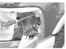
**STEP 4** Remove the 2 screws behind parking lights. The grille shell will be free at this point.
