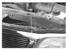
**STEP 2** Then remove the 6 screws from the top of the grille shell.
