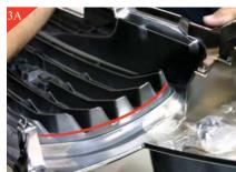
Lay grille shell face down, and using cut-off wheel or hack saw trim the remaining plastic.
