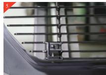
Next attach the Short "L" brackets to the bottom of billet grille as shown. The long end attaches to billet grille with U-Clips and #8 x 5/8" Phil Pan head screw.
