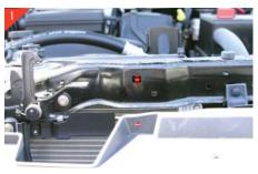
Remove the factory grille shell from vehicle, by releasing the (4) key hole tabs across the top of grille shell. Then there are (2) clips behind the parking lights on the driver & passenger side of grille shell, release by pulling straight out on shell. Then release (3) clips along the bottom of grille shell, by pulling straight out on shell.
