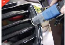
After grille shell is removed place shell face up on a protective surface, such as a blanket or rubber mat. Next you will be removing the center section of the factory grille shell, using a cut-off wheel or hack saw. Trim all vertical & horizontal plastic holding center in place.
