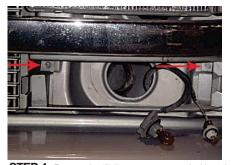
**STEP 4** Remove the (2)-7mm screws on each side at the back of the parking light housing as shown above. After grille shell is removed using masking tape–tape front of grille shell to protect chrome and painted areas.
