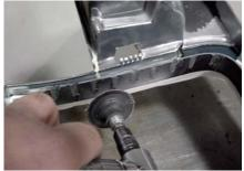
**STEP 7** Using a grinder or sanding block, smooth the cut surface flush with the sides of the grille shell.
