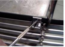
**STEP 9** Insert and center the billet grille as shown with the short edges of the brackets even with the back edges of the shell, then clamp in place and mark the slotted hole locations and drill a 1/8" hole 1/8" from the edges of the plastic on the center line of the slotted hole.
