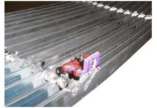
**STEP 8** Attach the long edge of the brackets to the billet grille using the supplied hardware as shown.
