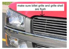
**STEP 5** Center the Billet Grill and make sure the front edge of the grille shell and the billet grille are flush as shown.
