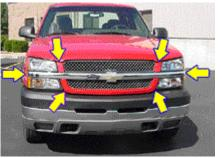
**STEP 1** Remove fan cover by removing plastic push rivets. Next remove factory grille shell by firmly pulling out on the 6 clips at each location shown above.
