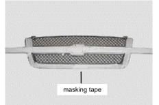
**STEP 2** Next tape off all painted or chrome areas using masking tape to protect the finish of the grille shell during installation.
