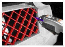
**STEP 3** Cut out the cross hatch area (shown in Red). On the top & bottom portions of the grille shell.
