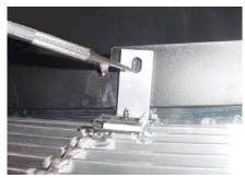
**STEP 5** Set billet grille in shell with back edge of grille sitting against black lip in shell and mark location of slot in 4 places. Then drill 1/8" holes and attach U-Clips to grille shell.
