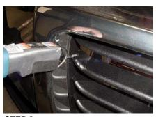
STEP 2 Using a cut-off wheel or hacksaw, remove the horizontal center bar section. Note: Do not remove the small black ring around the perimeter of the shell.
