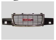
**STEP 1** Remove stock grille shell form vehicle. Next tape off chrome areas to prevent any scratching of the stock grille shell during installation.
