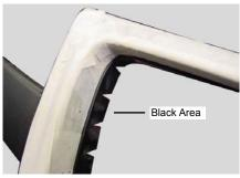
**STEP 3** Grind or sand ring around perimeter of the shell smooth. Note: Be sure not to cut the black area away as shown above.
