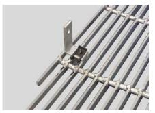
**STEP 4** Attach brackets to billet grille by using #8 x 5/8" Blk. Phillips head pan screw & U-Clips. As shown above.
