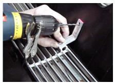
**Step 5A** Attach mounting brackets to the top grille section as shown, mark and drill (2) 1/8" holes through the top of the factory gille shell. Attach the top brackets using the black #8 x 5/8" screws and U-Clips supplied and Re-install grille.
