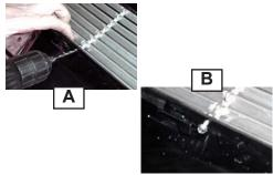
**Step 5** Center Billet grille into openings and clamp in place. Mark and drill 1/8" holes in center of rod locations for the bottom rods in the top section and both top and bottom rods in the bottom section (REF A). Reinstall the billet grille into the shell and attach using the #6 x 1/2" self tapping screws into the ends of the grille rods (REF B).
