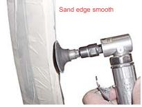
STEP 6 Carefully sand edges as shown above. Use a flexible sanding block with 240-320 grit paper to smooth remaining rough areas of the shell.
