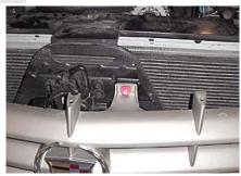
STEP 2 Remove the 10mm. bolt as shown above.
