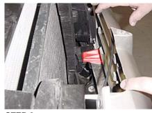
STEP 3 Pull out on upper left & right corners of shell to release the two upper clips. Then pull up on lower corners to release brackets.
