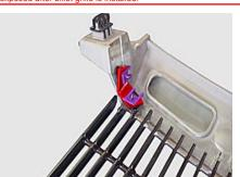
STEP 7 Place grille in shell and attach brackets to top of grille to match shell. Mark hole locations and drill 1/8" holes and attach using #8 x 5/8" screws.
