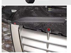
STEP 1 Remove core support cover by lifting the 8 plastic pop rivets, shown above.
